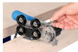
Thread the chain through the tool position first link on rivet pin Set counter to zero
